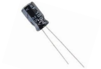
100 \mu F capacitor (Polarity)
